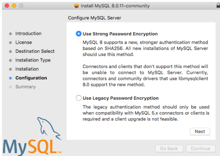
Figure 2.22 MySQL Package Installer Wizard: Choose a Password Encryption Type
