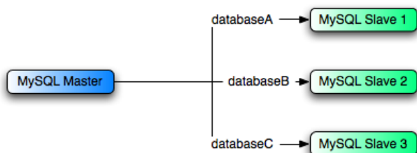
Figure 17.2 Using Replication to Replicate Databases to Separate Replication Slaves
